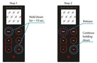
Then let go of "ESC". The bootloader splash screen will appear on the remote control screen, and a new device will appear in Windows Explorer, where you will see a readme file with hints and an Internet shortcut, which will take you to the page with the description of the remote control and firmware:
